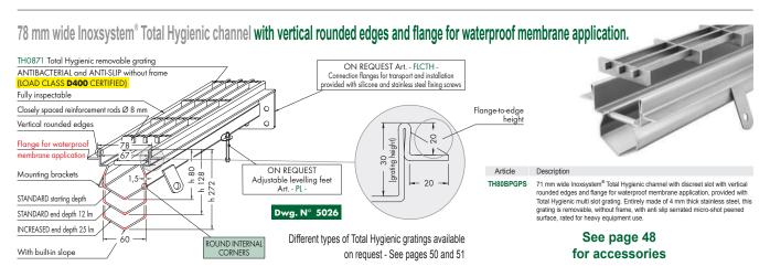
Dimensions can be modified on request - heavy duty top covers made from 6/8 mm thick stainless steel plate These technical drawings are property of INOXSYSTEM<sup>®</sup> and cannot be copied or reproduced without our prior written permission Page **49**
